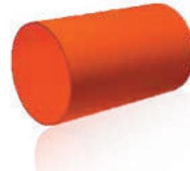
WS Intermediate Sleeves are used in conjunction with Link-Seal® Modular Seals to seal all pipes passing through concrete or masonry structures that require two belts of seals to fill the annular space between pipe and wall. Please see page 21, sealing an oversize annulus.
