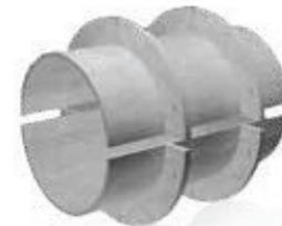
Model WS Split Sleeves are used for installations where an existing pipe run needs to penetrate a wall yet to be constructed. During wall installation a split sleeve is welded around the existing pipe and positioned in the form to center the pipe. After installation a Link-Seal® Modular Seal is used to seal the annular space between split sleeve and pipe.
