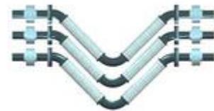
Unlike large pipe loops, Uni-Loops take up a minimum of space, providing pipe motion accommodation solutions in limited space situations such as indoor piping. The small configuration of the Uni-Loops are also far less susceptible to the heat loss that must be dealt with in the case of large pipe loops.
